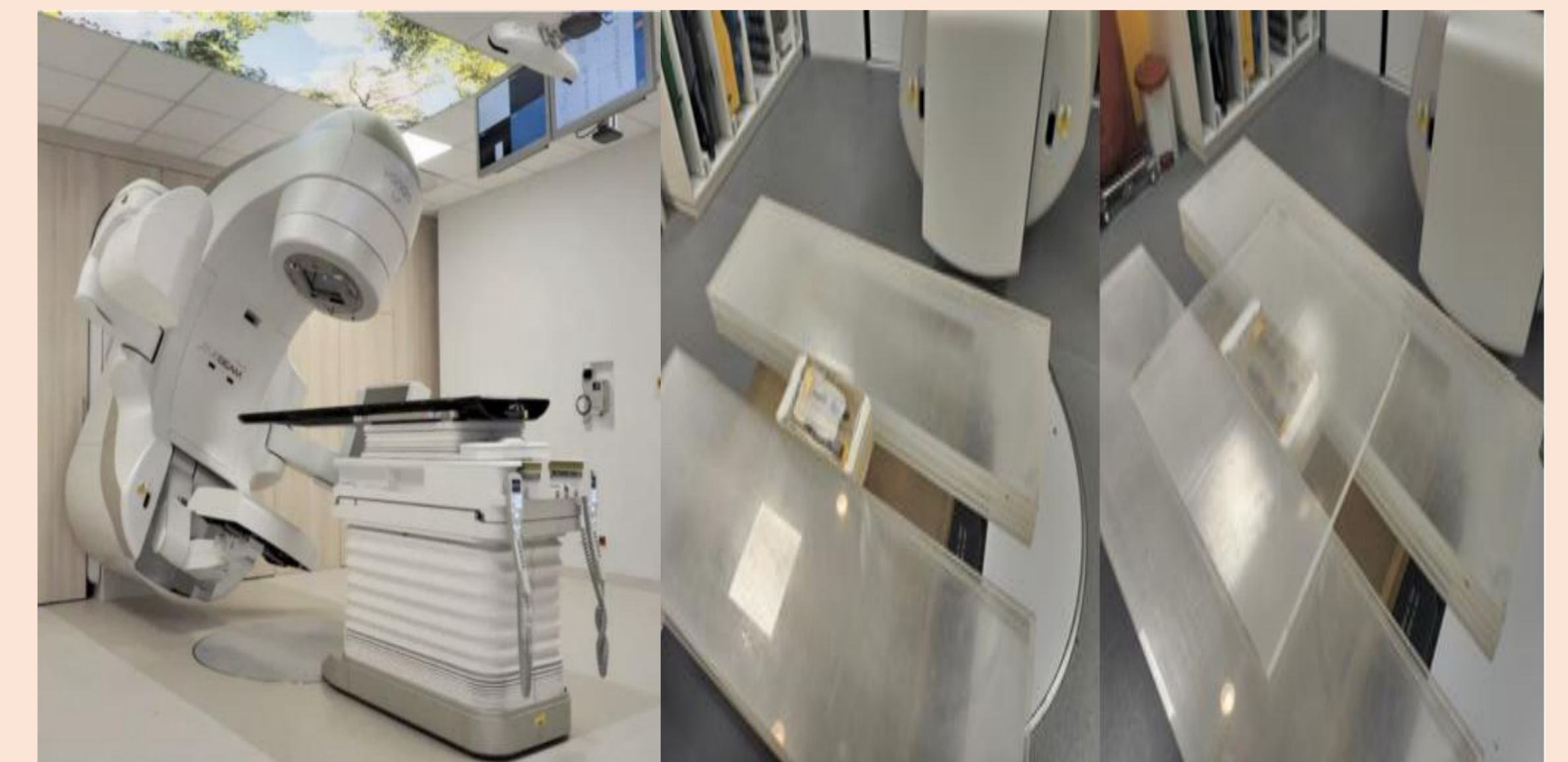
LINAC Accelerator with self designed phantom for cells irradiation
